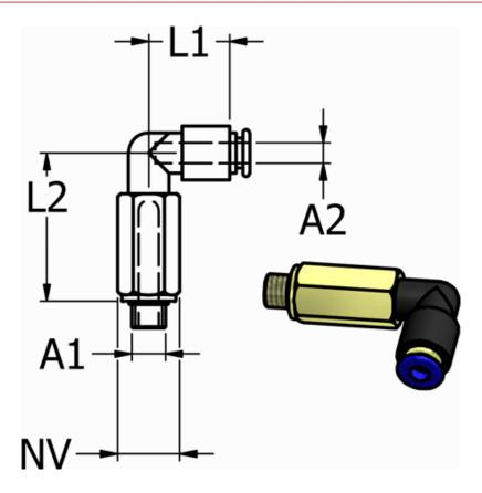
Ext. hose diameter A2 = 4 mm L1 = 28 L2 = 17.2 NV = 8 Thread A1 = M5
